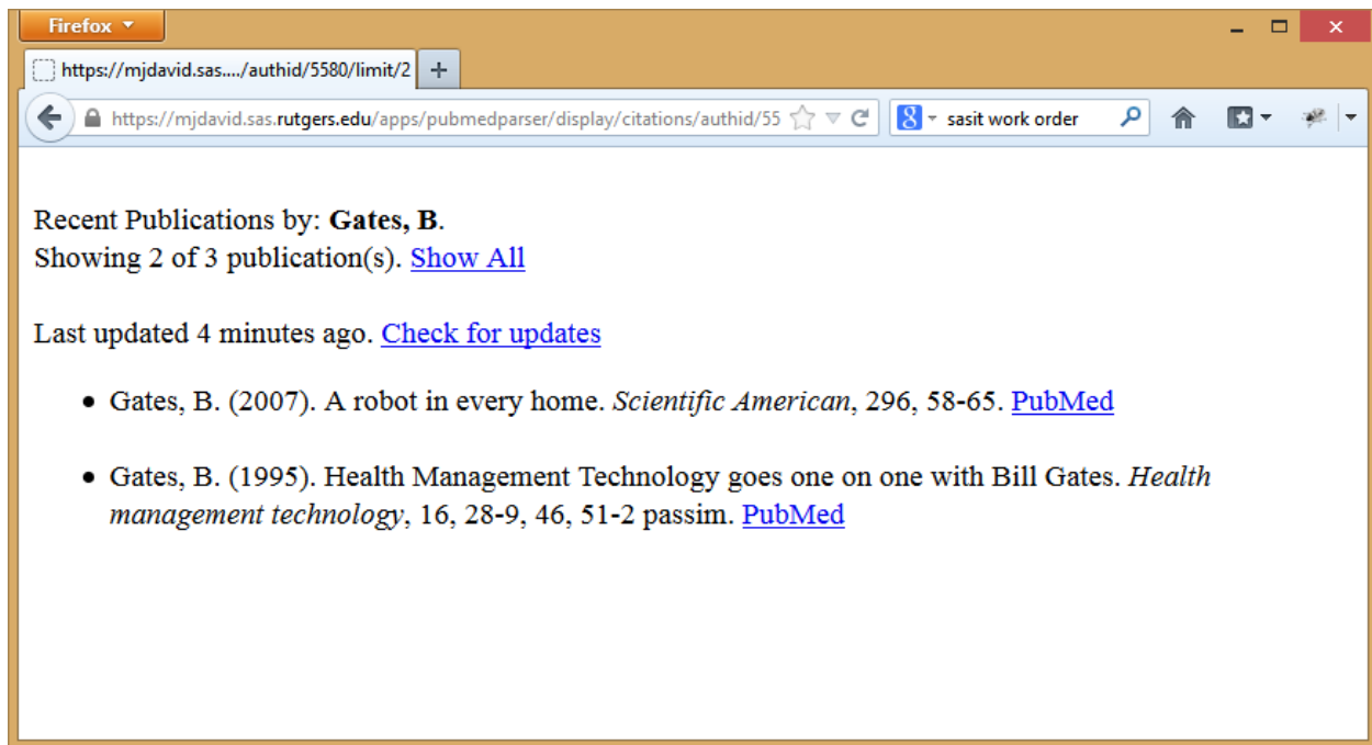
Figure 7-3 Example of limitation of returned publications Notice that the limit of two articles has been applied. The end-user has the ability to display all publications by clicking “show all”. If an invalid limit is given, then the iframe behaves as if no limit was given at all.
